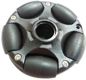
With the help of omni wheels, robot kit can move to all direction.
